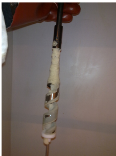
Figure 15 Hydrate growth on drill bit (used for stirring) when salt (35‰ of water mass) was added to the solution of 80 % cyclopentane (by weight) and 20% water.
