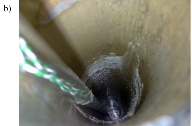
Figure 17 Hydrate experiment running 20% cyclopentane and 80% water. a) Measured attenuation and temperature. b) Drill bit covered with hydrates. The hydrates froze solid in this experiment.
